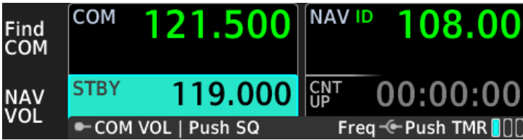
Timer is grayed out until you activate the function. Count up (CNT UP) is the default timer selection.
